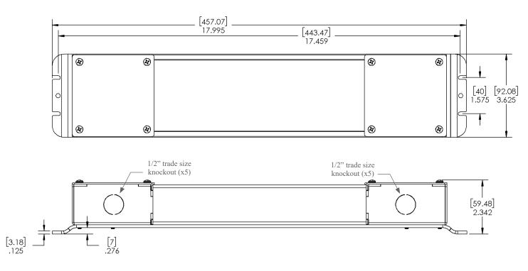
Mounting dimensions: 480W, 600W 24PS HLG Power System
