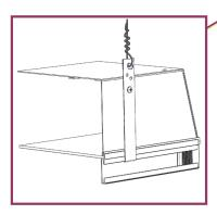
Insert the assembled fixture into the grid much as you would a ceiling tile.
