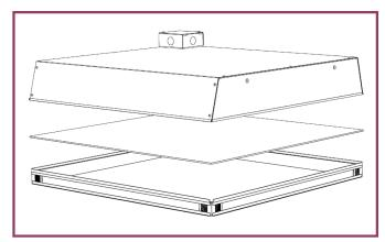
Use the hanger brackets to secure the Elevator to the light box.
