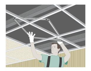
Next, drop the SkyTile into the Elevator.
