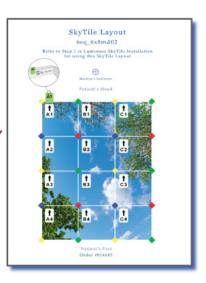
Check SkyTile Layout for proper placement of elevator with Sky Factory logo
