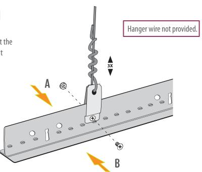
Note: Where possible, do not hang adjacent runners in the same 2' x 2', 60cm x 60cm, or 62.5cm x 62.5cm opening: installation of the fixtures may require one open side above the grid into which they can be temporarily inserted before dropping down into the grid pocket.
