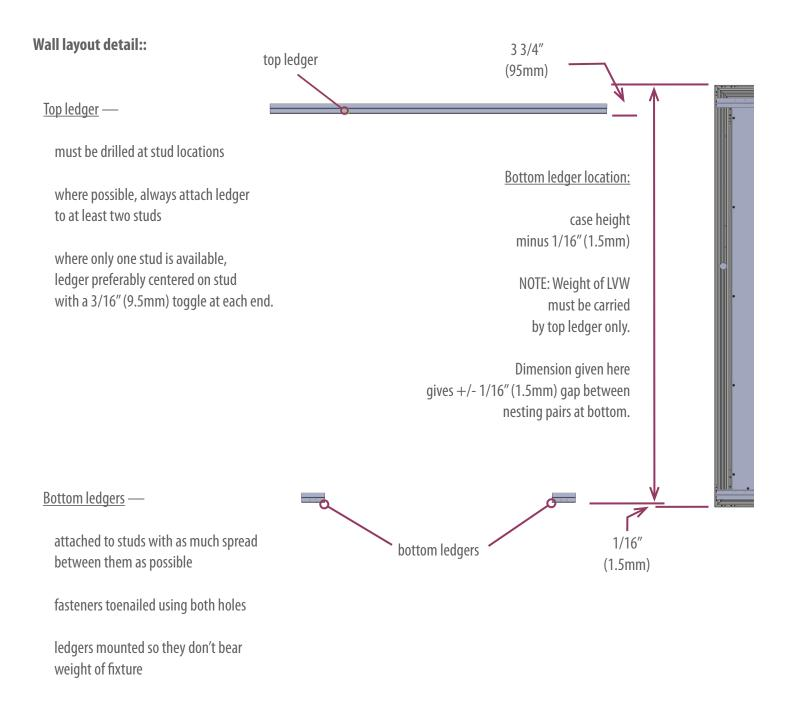
IMPORTANT: Ledger brackets must be mounted <u>flat</u>, <u>plumb</u>, <u>square and dimensionally accurate</u>.
