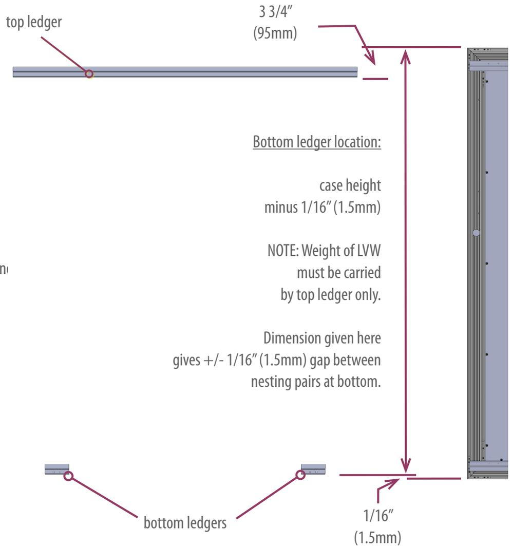
**IMPORTANT:** Ledger brackets must be mounted flat, plumb, square and dimensionally accurate.
