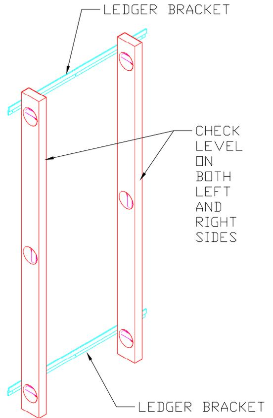
Bubbles on the builder's level must read the same for both vertical sides.
