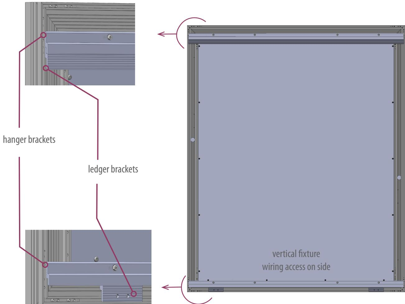
“Ledger” brackets are client-mounted on the wall:
