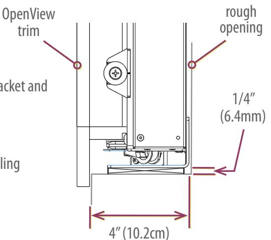
Brackets have 1/4" slots for fine adjustment and 1/4" diameter holes for final attachment.
