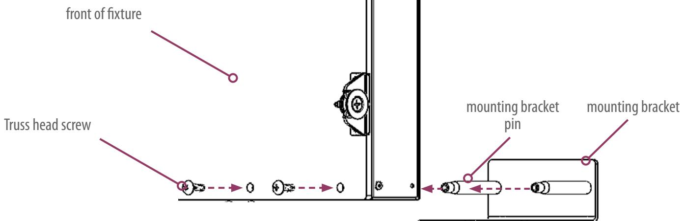
Insert the two pins of each bracket into the two holes at the bottom and top corners of the light box.
