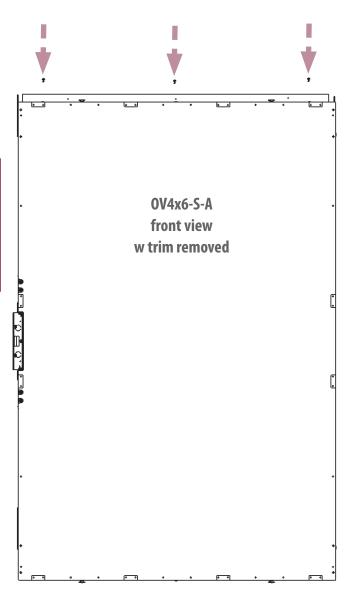
7. Then set fixture on bottom mounting bar and while one installer holds fixture in place, second installer secures it to bar with at least two fasteners.
